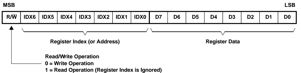
Figure 24. Control Data Word Format for MDI
